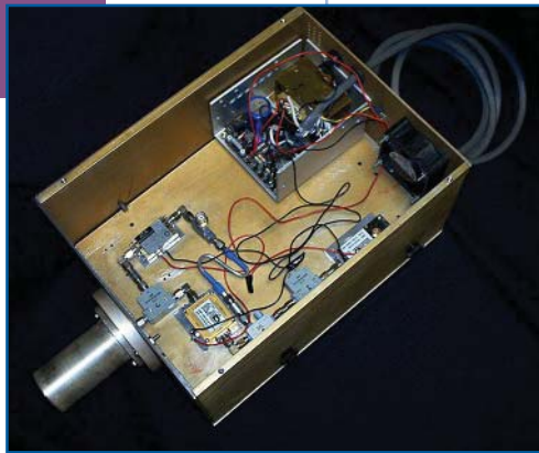
Prototype. Sentor’s radiation detector should provide high energy resolution, operate at room temperature, and have a large working volume.
