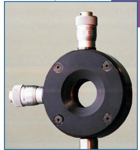
Beam tweaker. MetaStable's beam director is manually controlled and uses simple screws or, for more precise applications, micrometers. This summer, company officials plan to introduce a unit with motorized controls.
