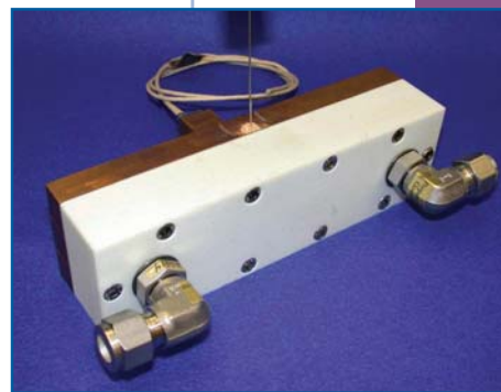
Copper pipes. Mudawar's thermal test module promises to remove up to 1,900 watts per square centimeter.
